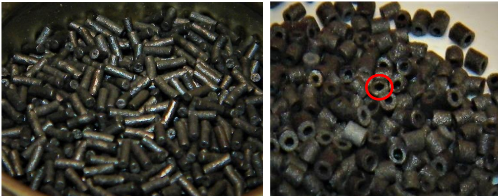
Figure 5: Single Perforation Tubular Propellant (IMR 3031 & Blackhorn 209)
